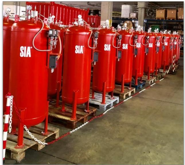
The FIRST AID RIM SEAL is a self-standing system, it doesn't need any external detection to be initiated or any external power to be activated.
